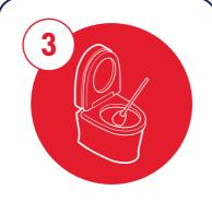
Reduce water level by pushing water repeatedly with brush
